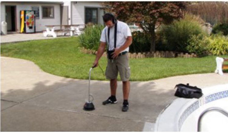
Figure 1 – Specialized Water Leak Detector 300-5000Hz in Use
